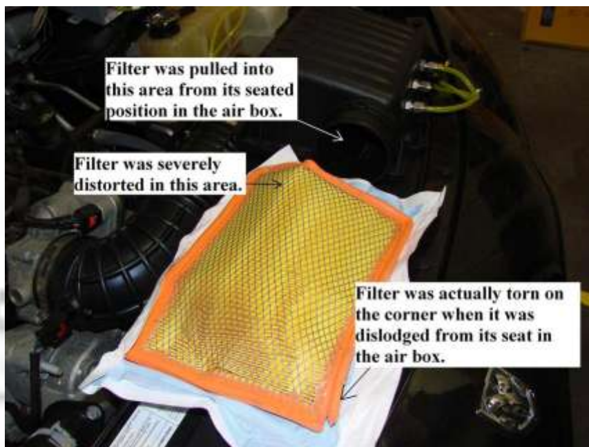
Fig. 3.6: Air filter damage from WOT testing 2008 Dodge Charger. Filter was damaged due to the pressure drop across the filter, resulting in the filter being torn out of its seat in the air box.
