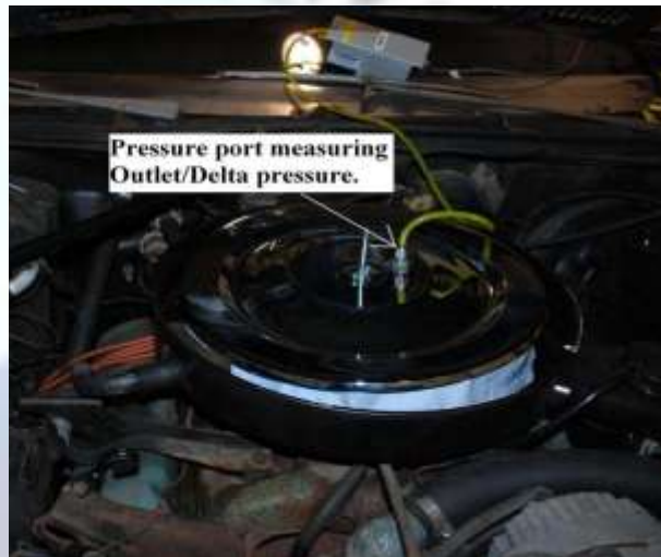
Fig. 3.9: Pressure port location for 1984 Super Saloon
