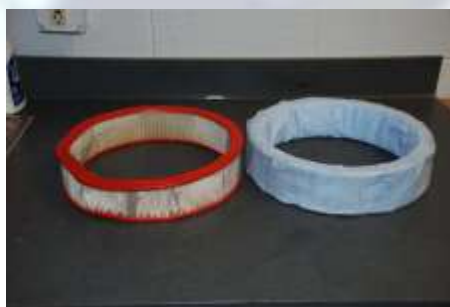
Fig. 2.6: 1984 Super Saloon air filter. Filter on the left shows damage that occurred during “severely obstructed” filter testing.
