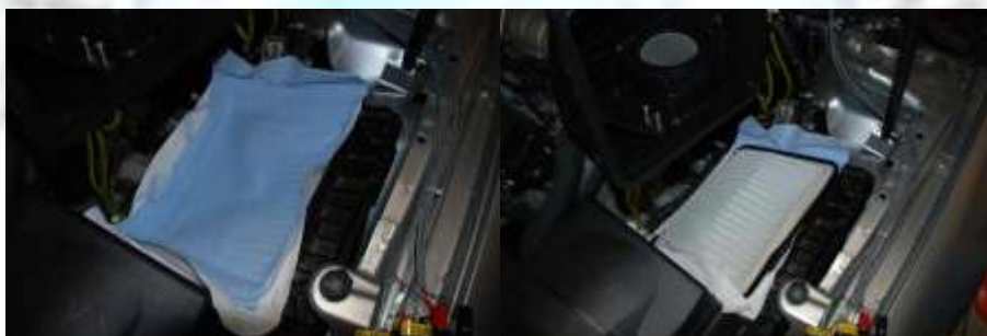
Fig. 2.5: filter restriction. Shop towels inserted into air box upstream of the air filter.
