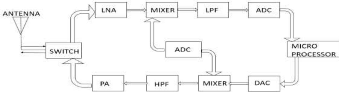
Figure 2. Block diagram of a transmitter
