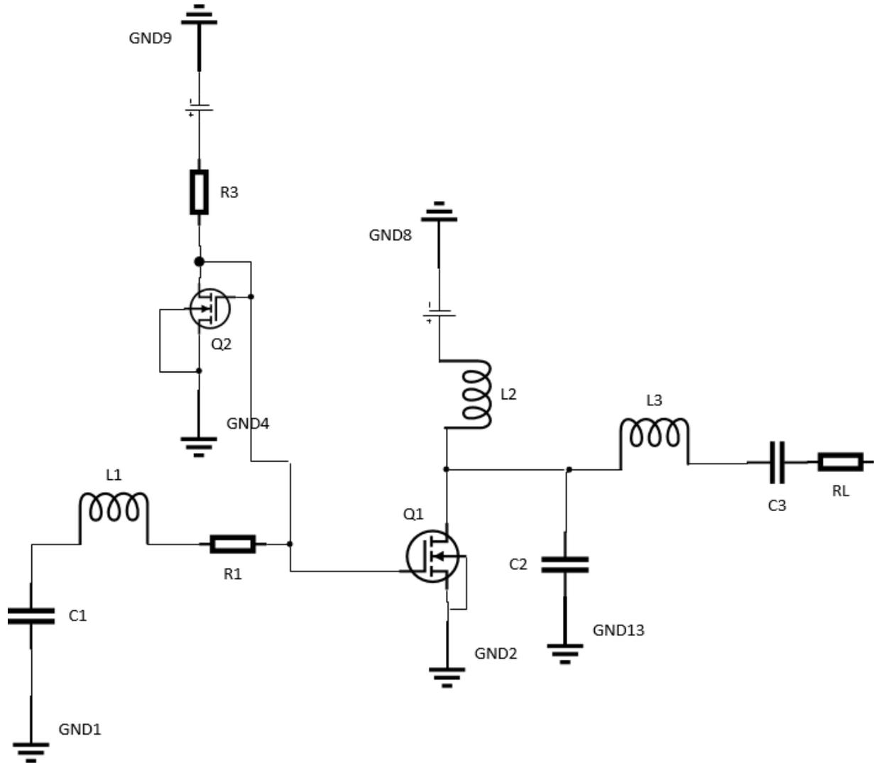
Figure 3. Block diagram of a single ended class E power amplifier
