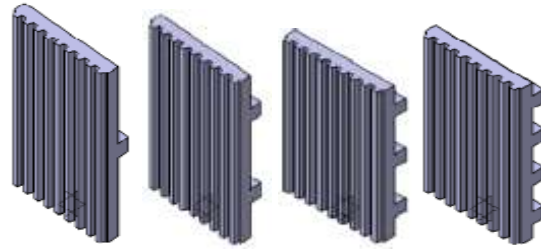
Fig. Swing Jaw Plates(1200X900X216) with Stiffeners
