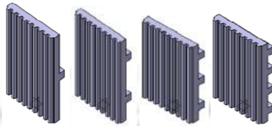
Fig. Swing Jaw Plates(1200X900X224) with Stiffeners.
