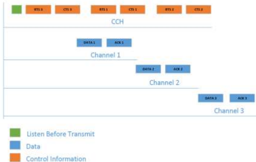
Figure 3. Flow of control and data information in the random access CR MAC protocol
