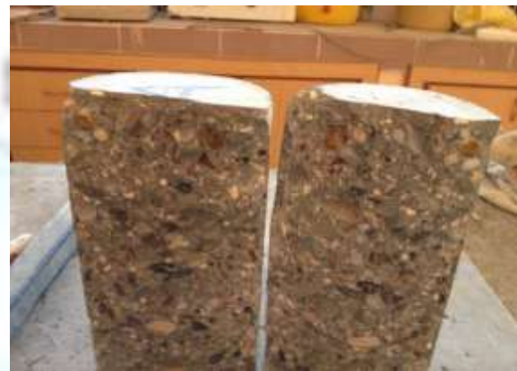
Figure 2. Tension failure concrete cylinder
