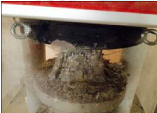
Figure 3. Concrete cube under compression machine
