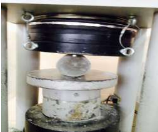
Figure 1: Cylinder tested for Splitting tensile
