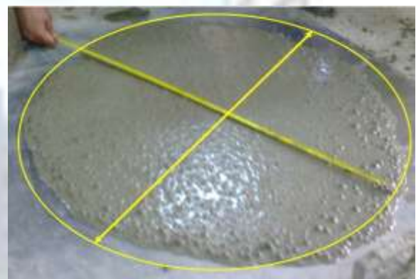
Figure 4. Photographic expression of slump flow diameter measurement
