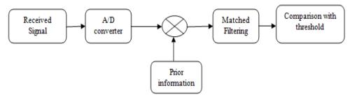
Input signal s(t) is passed through A/D converter to get discrete time signal s(n). This signal further multiplied with prior information  $s^*(n)$ . [12]
