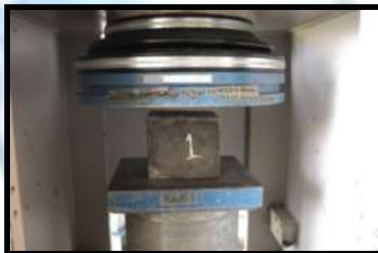
Figure 1: Compressive strength test procedure
