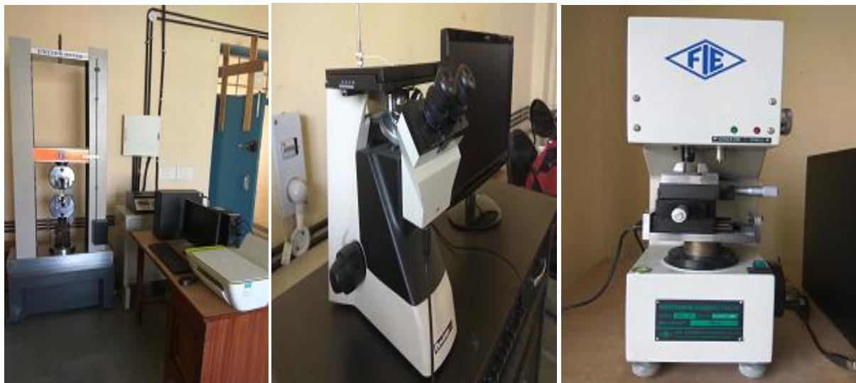
Fig. 5: a) U.T.M Unitek 94100 b) Microstructure Tester c) Microvickers Hardness Tester
