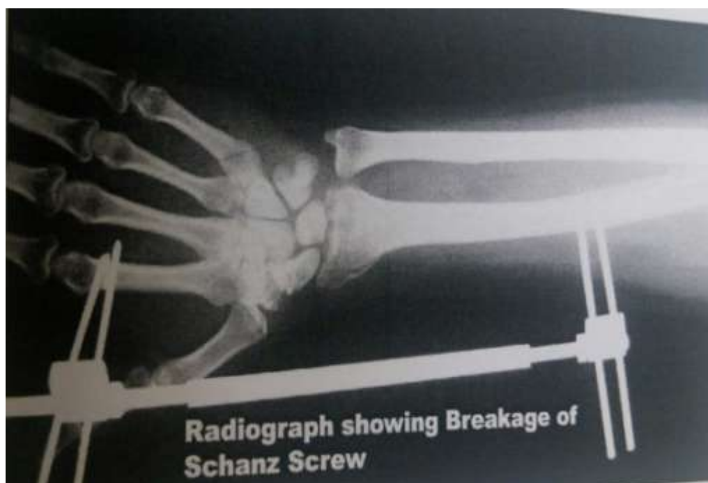
Figure 3: Radiograph showing breakage of schnaz screw
