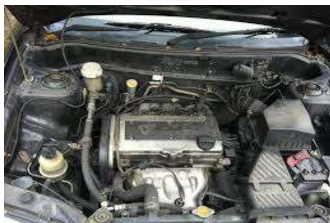
Fig. 3: Air box system located under the bonnet of proton wira
