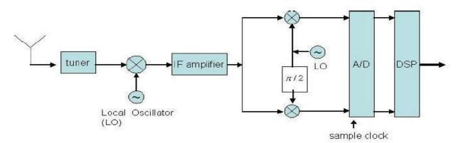
**Figure 5.1 OFDM Receiver Front End**
