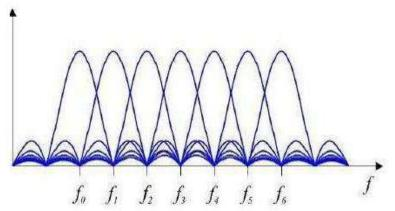
Figure 1: Bandwidth utilization of OFDM.
