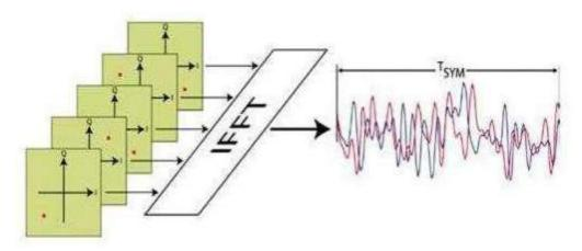
**Figure 2: Transmitter implementation using IFFT**
