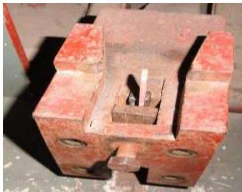
Fig-1: Sample is placed vertically with notch facing towards the pendulum for Izod impact test
