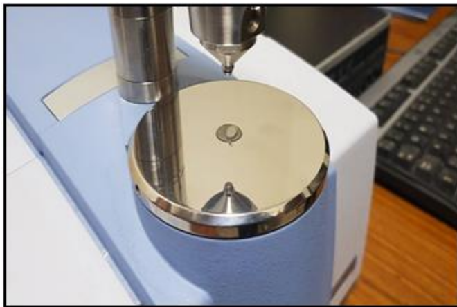
Figure 5: Sample placement on FTIR testing table and lens.
