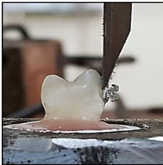
Figure 3: The SBS testing in Universal testing machine with a knife edged blade
