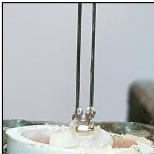
Figure 4: The TBS test via S.S. ligature wire of 0.010 gauge.
