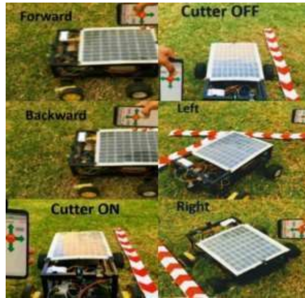
Figure 5: Different Movements of Grass Cutter The final demonstration of the proposed grass cutting robotic system with four different types of pattern like Circle, Spiral, Rectangle and Continue shapes designing on the grass is as shown in Figure 6.
