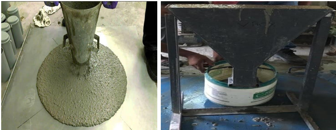
Figure: Fresh Property Tests Slump Flow [1] and V-Funnel [2]
