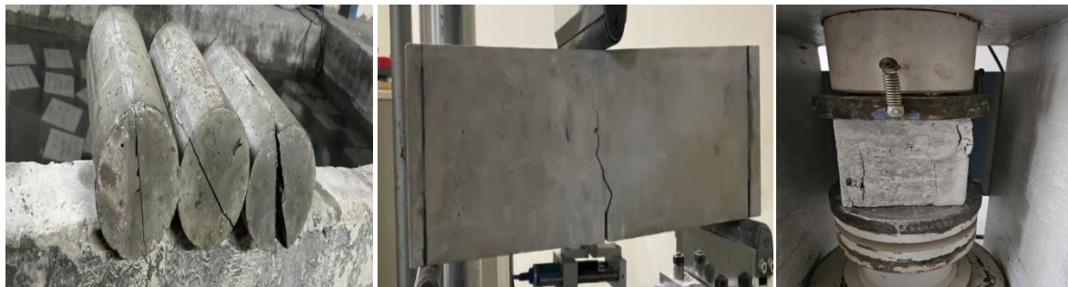
Figure: Specimen Failure Modes Plain SCC vs. Jute Fibre SCC at RT and 200°C
