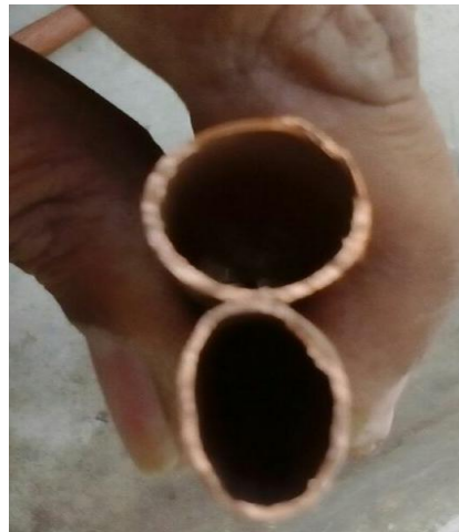
Plate 3 Circular and Oval Pipe
