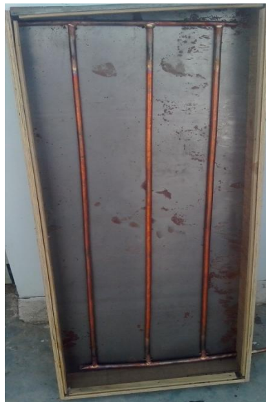
Plate 1 Solar Water Heater Assembly
