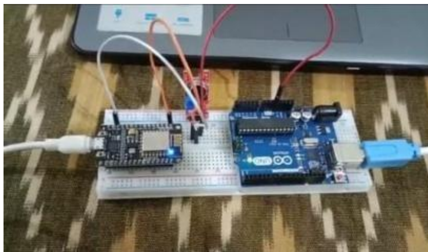
Fig. 1 Noise level detector using arduino and a sound sensor
