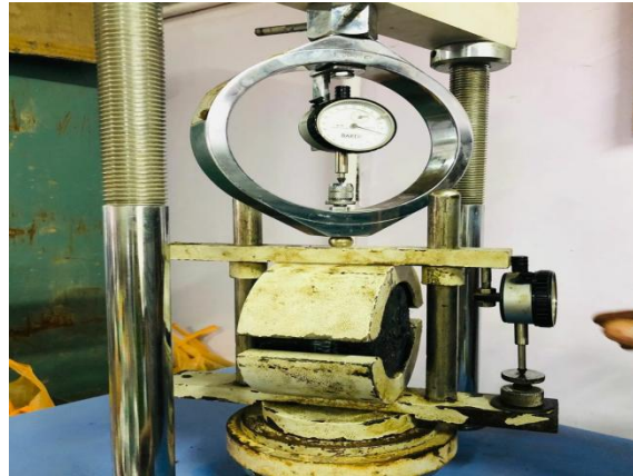
Figure 03, Marshal Stability test
