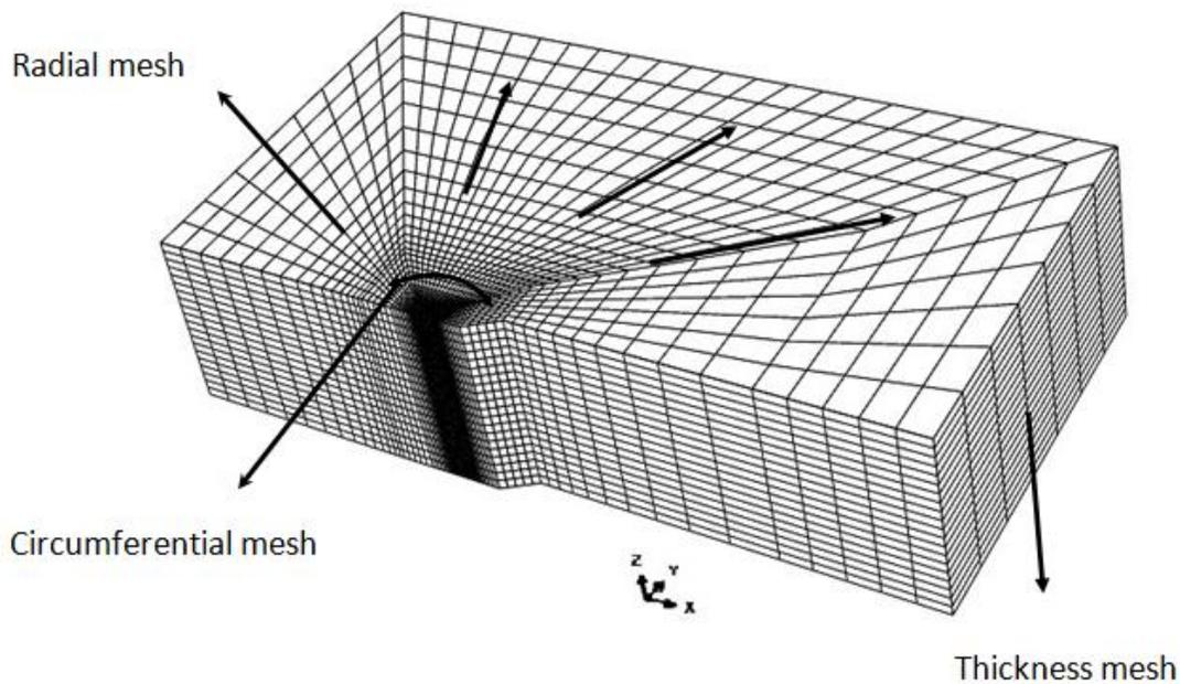
Fig 1. Half CT specimen with final mesh in thickness, radial & circumferential direction
