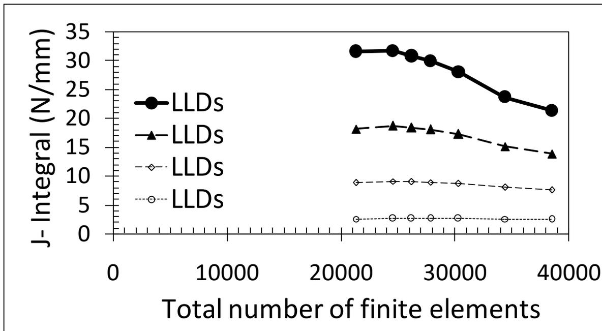
Fig.3 variation of J-integral with element variation in radial direction
