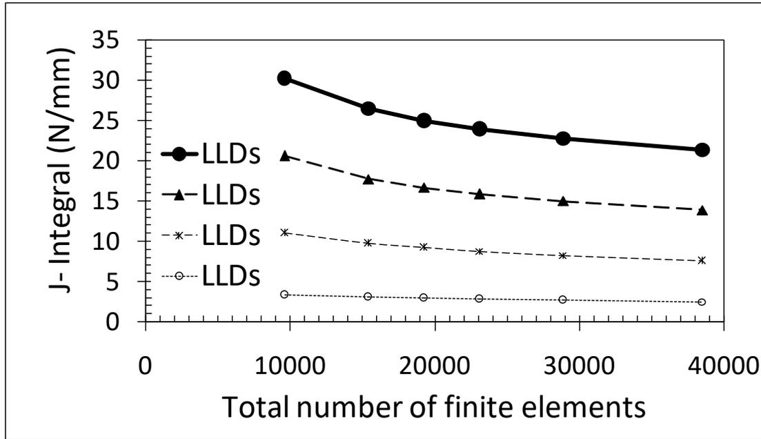
Fig.2 variation of J-integral with element variation in thickness direction
