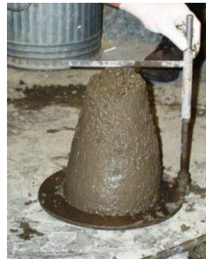
Fig. 2. Measuring Slump Fall
