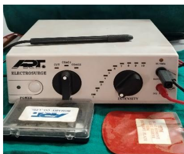
Figure 3: The electrosurgical unit
