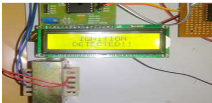
Figure.10: The Ignition Detected Message Display.
