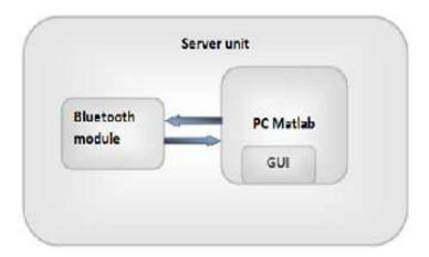
Wireless data acquisition system comprises of two parts, the part of the data acquisition and the part of the data processing in the host computer. The data acquisition part of the sensor circuit handles the important task of receiving the external signals, and these changeable signals can be amplified through the amplifier circuit. Sensor circuit includes GAS sensor, Humidity sensor and temperature sensor. Gas Sensors are from MQ Series .The amplified signal will undergo a process
