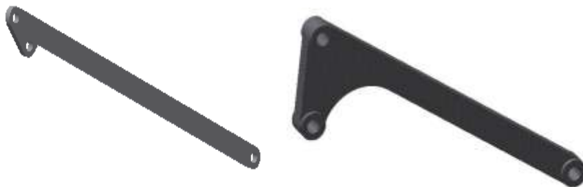
Fig. 6.2: The comparison of original and modified upper rocker
