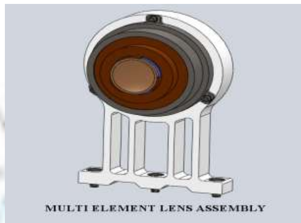
Fig 3.1: Geometric model of multi element lens assembly
