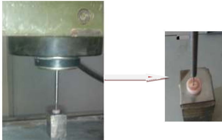
Figure (3): Loading Performed Using a Computer Controlled Universal Testing Machine ( Afa,UK)
