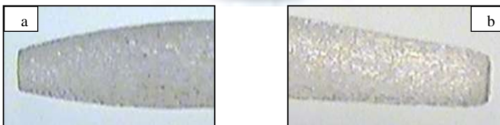
Figure (2): The Surface of the Fiber Post Under Stereomicroscope X20. a: Before Treatment, b: After Laser Treatment.
