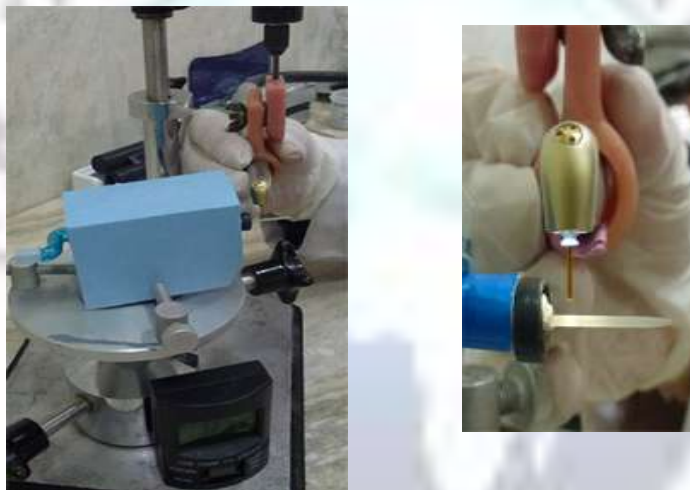
Figure (1): The Fiber Post Fixed in Mechanical Rotator Horizontally.
