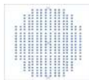
Figure 4: Schematic design of mask 2 on chrome glass
