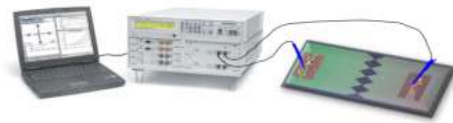
Figure 9: Capacitance measurement set up with a dielectric analyzer
