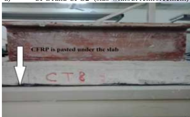
c) CPG4 (slab under tension with CFS reinforcement)
