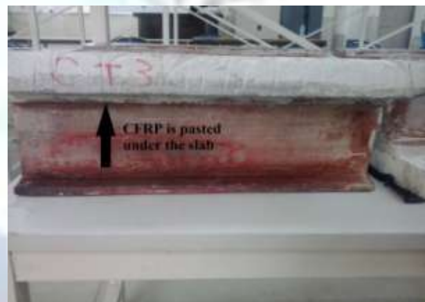
b) CPG3 (slab with CFS reinforcement)
