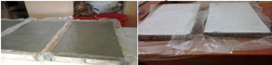
Figure 4. Casting and removed concrete slabs from molds
