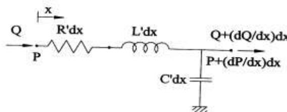
Fig. 2: Model of a line of length dx
