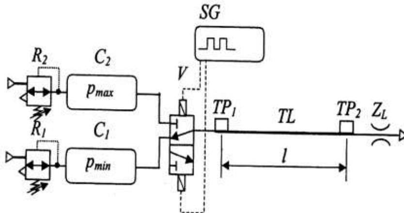
Fig. 4: Transmission line test bench
