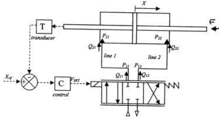
Fig. 1: Schematic view of a pneumatic servo system
