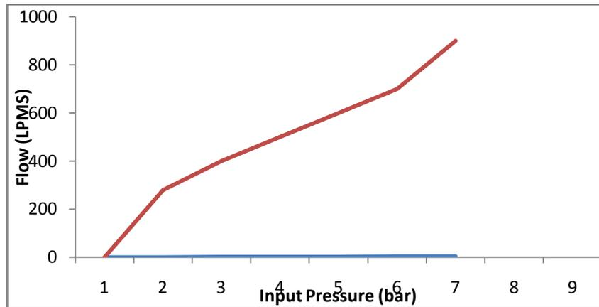
**Fig.8: The variation of flow with input pressure for line of length = 5 m and diameter of 5.5 mm**
