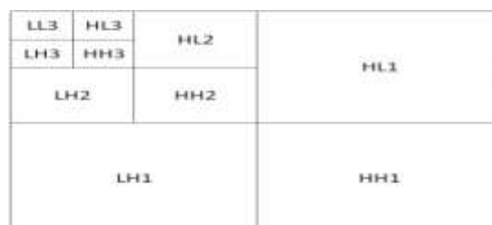
Figure 2: Three level decomposition of 2-D DWT coefficients
