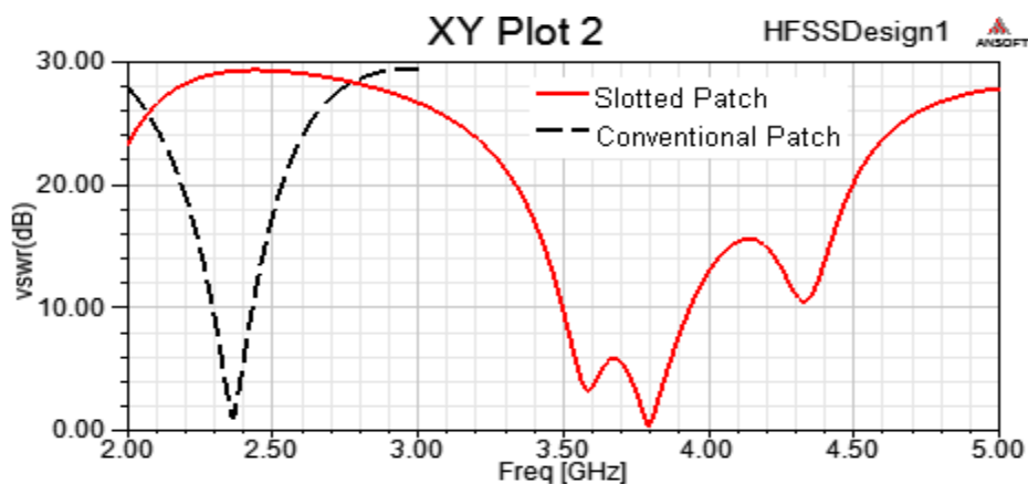
Figure. 4: VSWR of conventional patch and slotted patch antennas
