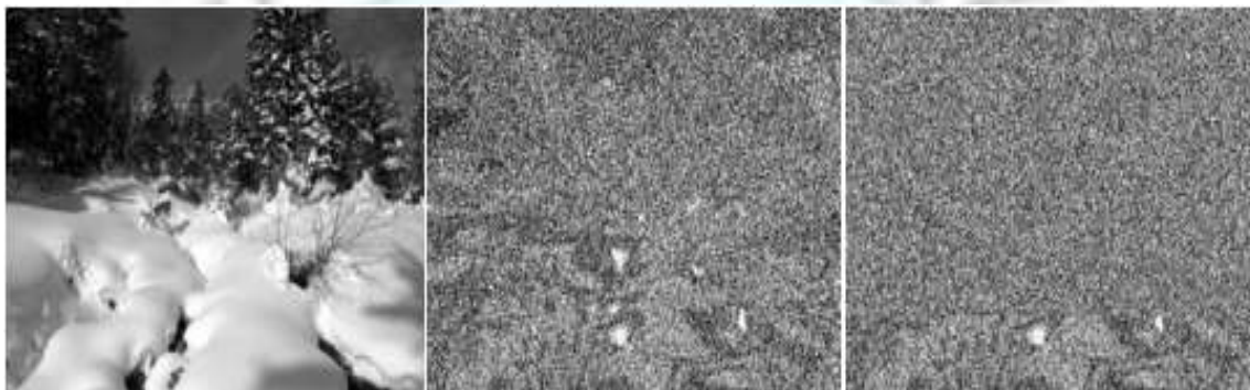
Fig. 3. Steganalysis using visual inspection: (left-to-right) original image, LSBs of the image before embedding and after embedding, respectively.
