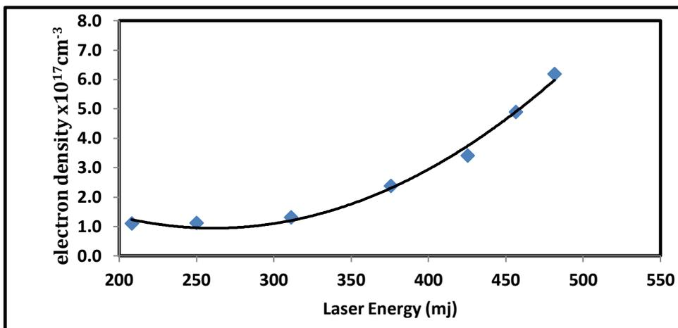
Fig 4: Variation of the electron density with different laser energy
