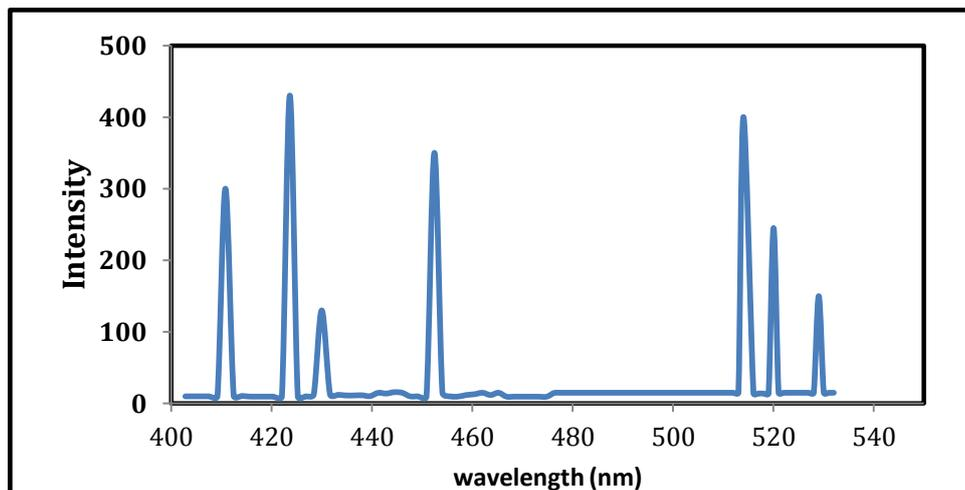
Fig.2: Optical emission spectrum of the Iron ablation plasma in air.
