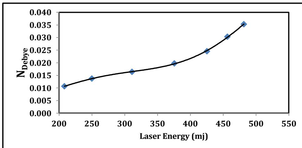
Fig. 6: Laser energy vs. number of particles in Debye's sphere.
