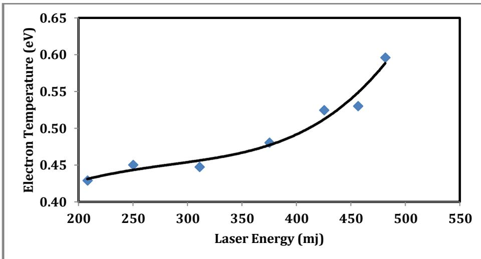
Fig 3: Variation of the plasma temperature of the plume with different laser energy
