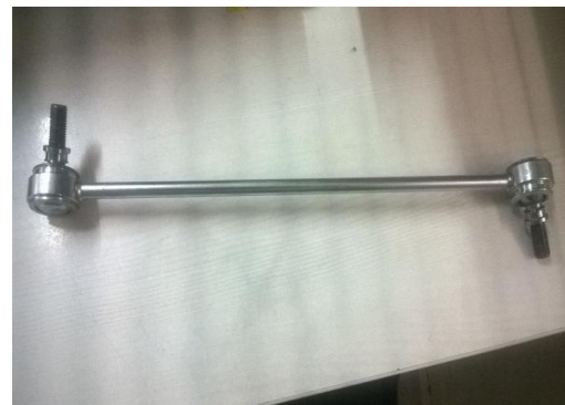
Fig. 5 Stabilizer Link Assembly
