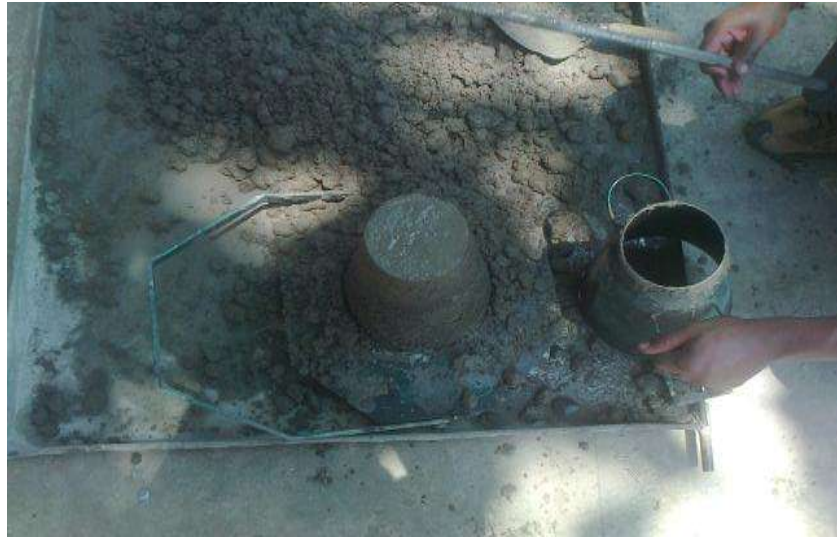
Figure showing the cone of the workability test
