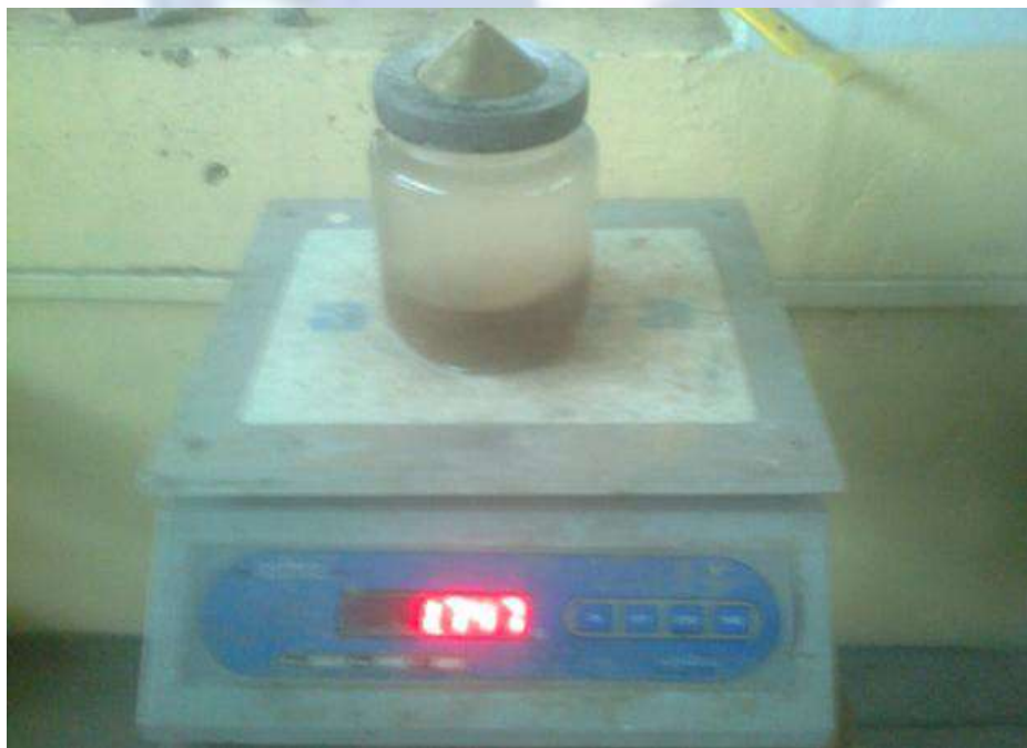
Figure showing the pycnometer with quarry dust, water
