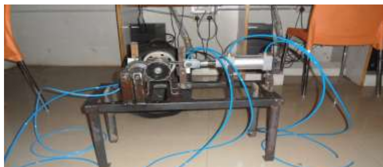
Figure 3 Prototype of the Compressed Air Engine
