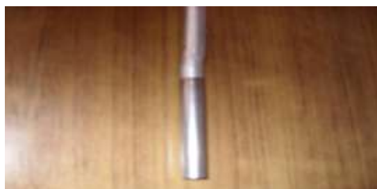
Figure 3.2 Friction welding of aluminium and stainless steel – 304
