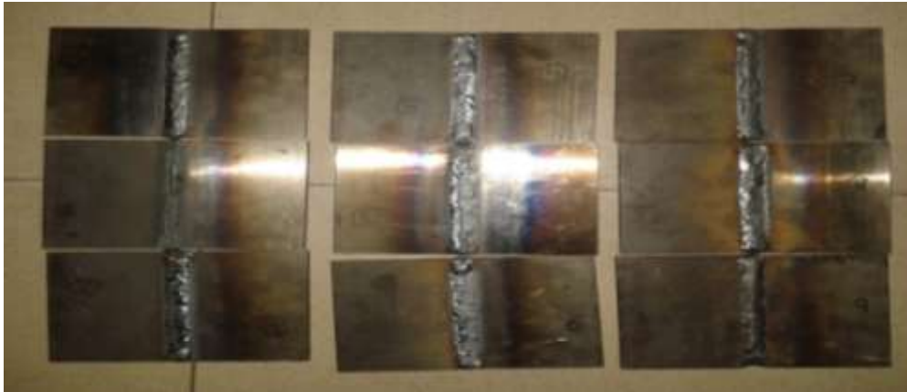
Figure 3. Weld Specimen after GMAW operation
