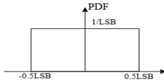
Fig. 3 Explanation of aliasing in frequency domain Fig. 4 Probability density function of quantization error [5]
