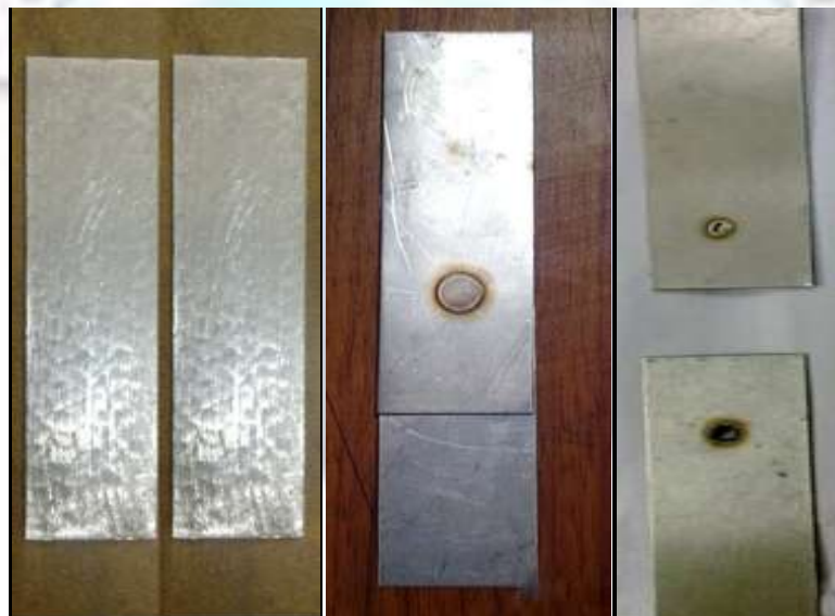
Figure 1: Workpieces before welding, after welding and after tensile test
