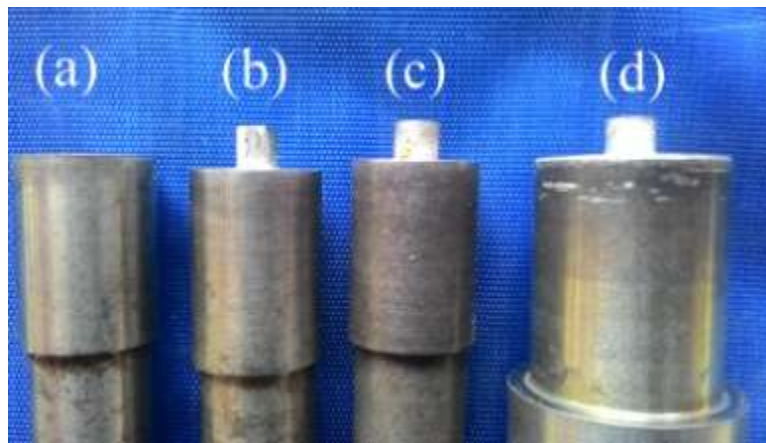
Figure 2. (a) pin less tool (b) square tool pin (c) cylindrical tool pin with 18 mm shoulder diameter (d) cylindrical tool pin with 22 mm shoulder diameter
