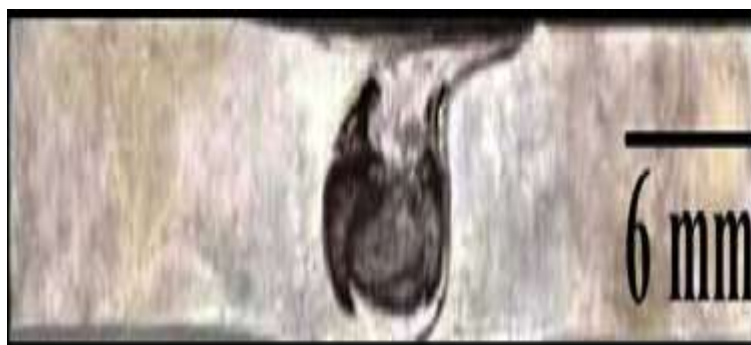
Figure 3. Macro graph of square tool pin profile /TiC MMC
