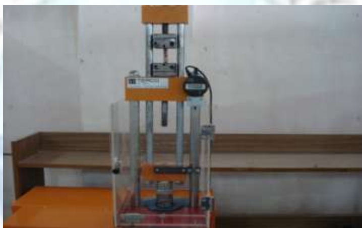
Figure (2): Terco universal testing machine.
