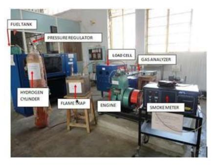
Fig.1: Photographic representation of the engine experimental set up
