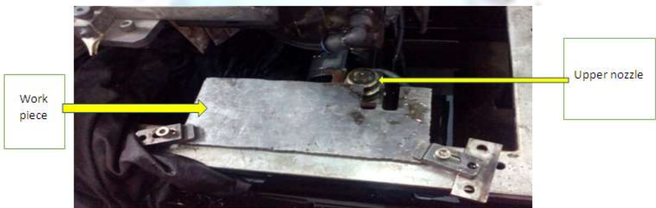
Figure 3: Clamping of the workpiece on work head of WEDM
