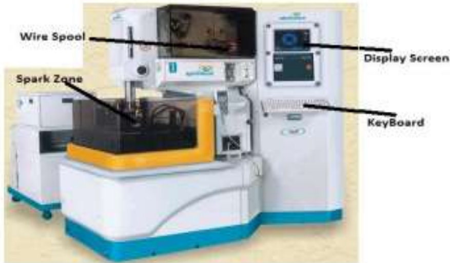
Fig. 2: CNC Wire cut EDM is used for experimentation
