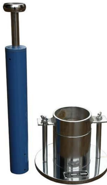
Fig. 2: Modified Proctor test apparatus
