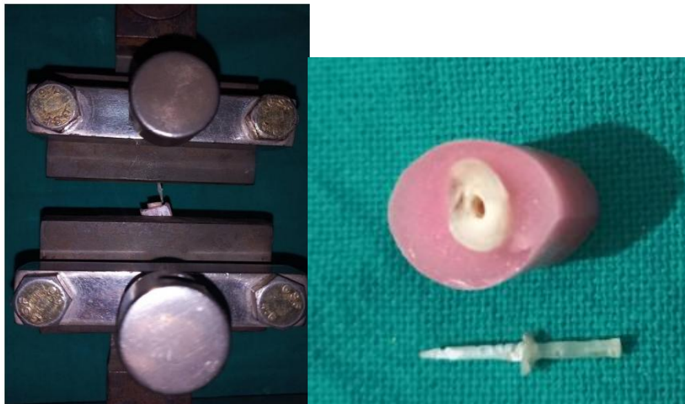
POST DISLODGED AFTER THE APPLICATION OF FORCE
