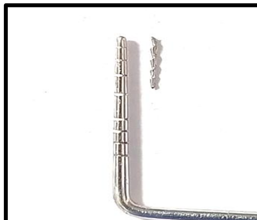
Figure 3) Fractured fragment of approximately 4.5mm in length
