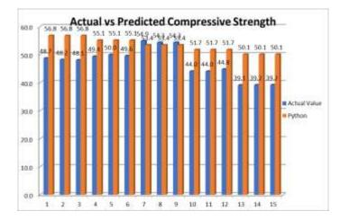
The actual values of concrete strength are derived from meticulous laboratory tests, conducted under controlled conditions, to ensure precision and accuracy. In parallel, predicted values are generated through the utilization of a regression model implemented in Python, a powerful tool for data analysis and modeling.
