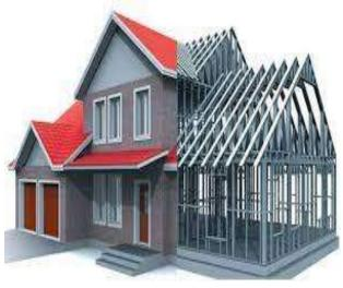
The LGS wall system comprises of a network of steel members connected to form a frame. The studs are connected to a top and bottom track to form a framed may depending on the load conditions, may also have bracing.
